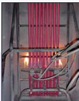
Bunched cables being tested for fire retardance .
